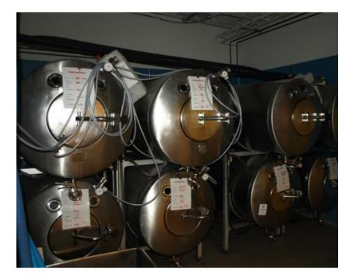
Fermentation of grape juice to make wine produces  $CO_2$  as a byproduct. Fermentation tanks have valves so that pressure inside the tanks can be released.
